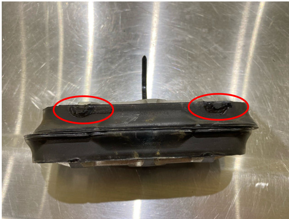
Figure 3.3.1 – Damage from Premature Wear
